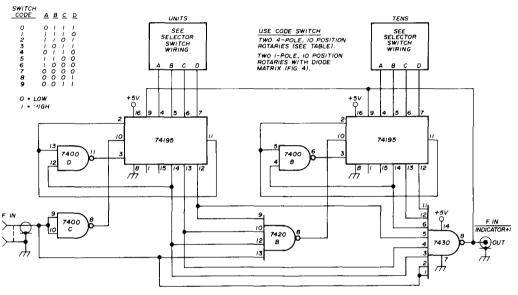
fig. 3. Logic for dividing by any number between 1 and 100. Circuit divides by one more than shown by selector switch (fig. 4), thus dials should be set at 00 to divide by 1; 09 to divide by 10; 29 to divide by 30; etc.
